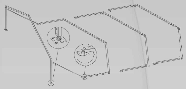
The assembly procedure for hoop one should now be repeated and the lifting gear transferred to hoop two so that it can also be hoisted into a vertical position.
